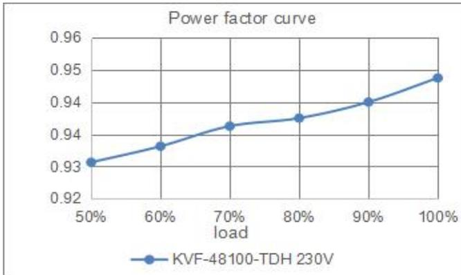
Phase cut /Triac dimmable driver-PWM output Dimmable LED driver 100W
